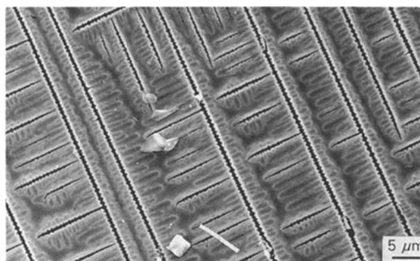
Figure 11 Oriented defects generated by the  $\text{NH}_4\text{Cl}$  dendritic crystallization and observed after thermal treatment ( $450^\circ\text{C}$ ).
