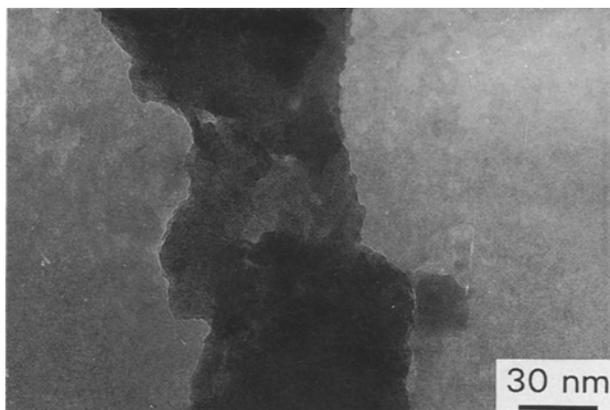
Figure 13 TEM observation of the homogeneous fine-grain texture observed outside the dendritic zones.
