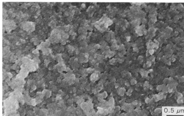
Figure 10 SEM micrograph of agglomerated  $\text{LaOCl}$  particles ( $A = 0$ ,  $B = 0.8$ ,  $C = 0.135 \text{ M}$ )
